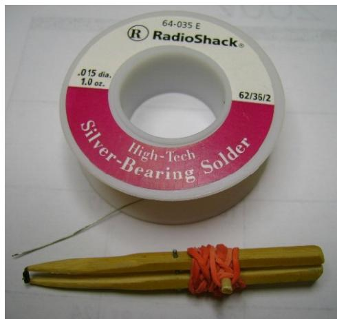
Surface mount soldering is best done with .015 dia silver-bearing solder. The tweezers used to hold the tiny parts for soldering is made from a bamboo chop stick. A web search will find lots of ideas for manual PCB assy.
