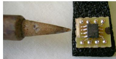
A soldering Iron tip shaped to a fine point. The tip shown here fits between the leads of an SOIC chip. Also allows soldering in close to the edge of parts that don't have extended leads, e.g., electrolytics, pots and some inductors, etc. Also makes it easier to solder chip capacitors and resistors. The soldering station is a Solomon SR-976 adjustable temperature.
