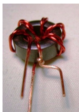
Leads formed ready for installation.
