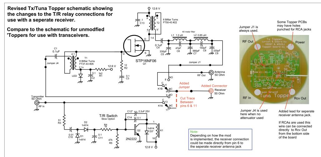
Make 2 cuts in the trace between pins 6 and 11 of the T/R relay. Strip out a short piece.
